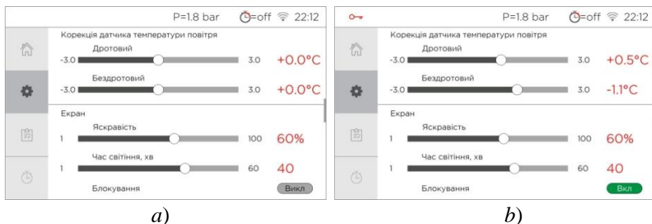
Figure 14.7 — The ‘Air temperature sensor adjustment’ and ‘SCREEN’ sections: a) — adjustment of the value of the air sensor, the brightness of the screen and its default glow time; b) — adjustment of wired and wireless air temperature sensors at +0.5 and -1.1, respectively, constant glow of the screen, the screen ‘ Lock ’ function is activated
